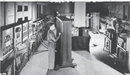
FIGURE 1.12.1 ENIAC, the world's first general-purpose electronic computer.
